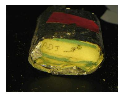
It doesn't have to be pretty. With scissors, cut off any extra AM and split end pieces enough to completely overlap the insulation and separate the wires. Notice the wires are coming out on the low side and indicating the bottom side of the OVB. This is a reference in the next step.
